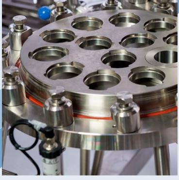
Additional microbiological stabilization stage construction details of the plate for cartridge mounting Safe system for filter closure.
